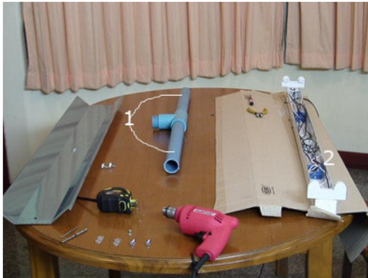
In this picture you can see our light is ready for assembly. We used 45ml pvc pipe as this fitted perfectly over the music stand I will show you later. We got a “T” piece and inserted 2 x 45 cm pieces (1). We then bolted this to the back of the fluorescent light case (2).
