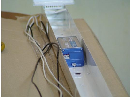
Slide the first fluorescent tube holder end piece (5) into the grooves at the end of the light fitting.
